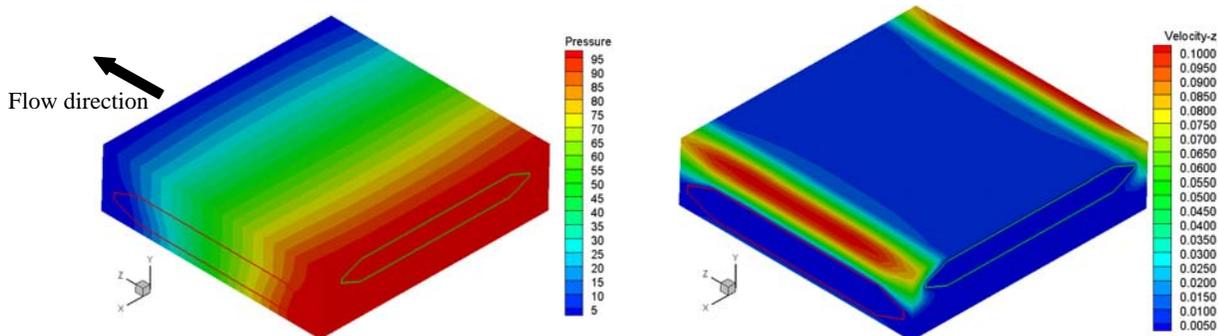
Fig. 6 Flow along the  $0^0$  direction of the small unit cell: (A) pressure contours; (B) velocity contours.
