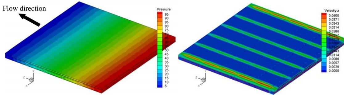
Fig. 4 Flow along the  $0^0$  direction of the big unit cell: (A) pressure contours; (B) velocity contours.
