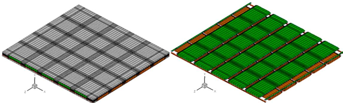
Fig. 2 Finite element mesh for the big (true) unit cell: (A) the whole unit cell; (B) just the fiber tows.
