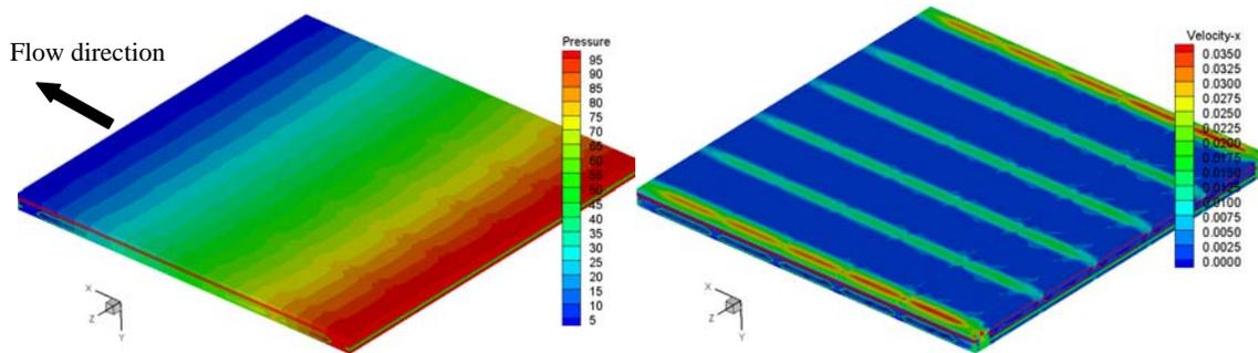
Fig. 5 Flow along the  $90^0$  direction of the big unit cell: (A) pressure contours; (B) velocity contours.
