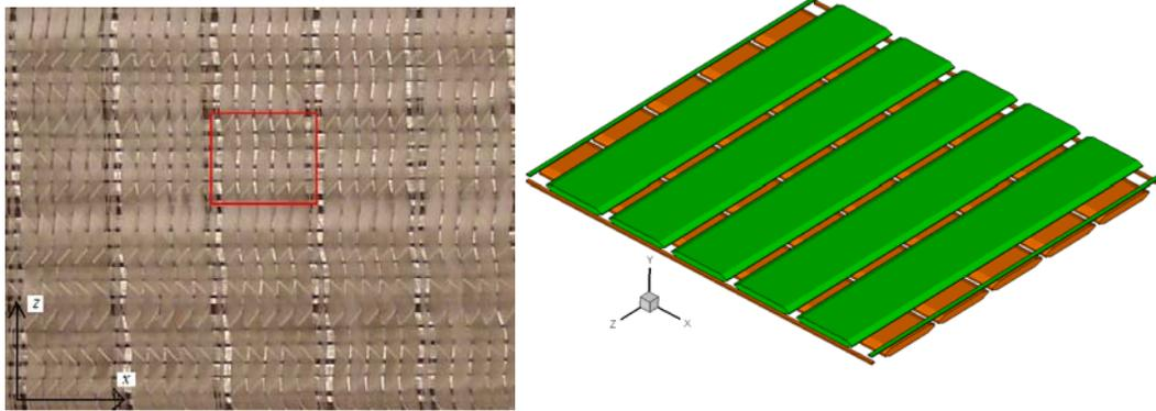
Fig. 1 (A) A photo of the biaxial fiber mat. (B) The big unit cell showing the two fiber-tow directions.
